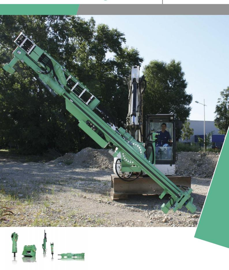
With CPA Montabert drilling attachment, your hydraulic excavator can be used for drilling as well as loading, trenching and demolishing.
