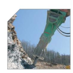
The hose swivel couplings are designed to ensure that the hoses can turn freely and avoid premature wear
