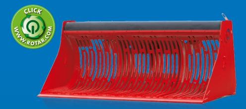
Two individually framed bar gratings are powered by a hydraulic motor, via an eccentric shaft, creating a reciprocating motion causing the under size materials to exit the bucket through the alternating bar spaces.
