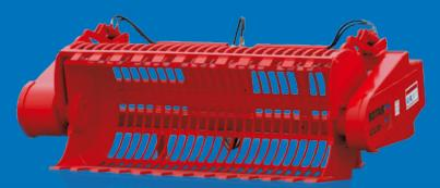
During the rotation, the fine's fall out of the drum and the bigger sizes stay in. By use of various sizes of changeable screens, different effects can be realized. With the rolling effect of the material, which stays in the drum, a cleaning reaction is realized by the scouring.
